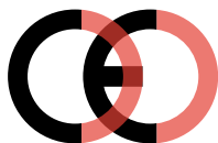
False CE Mark (too close)
