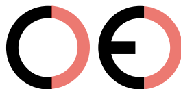
False CE Mark (too far)
